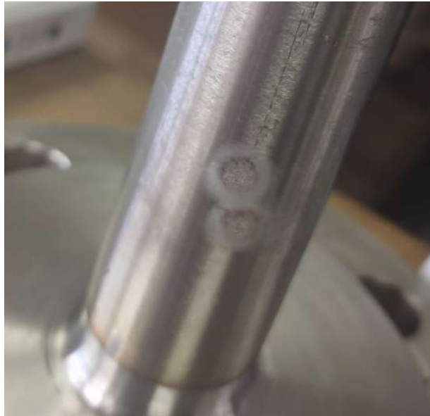
Fig.3. “Burn” Area on Stainless Steel
